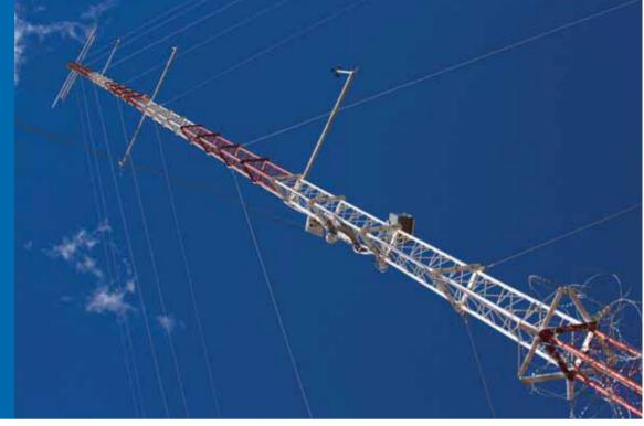
Close-up of a Wind Measuring Mast
